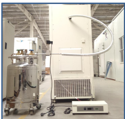
LN 2 /CO 2 backup system
